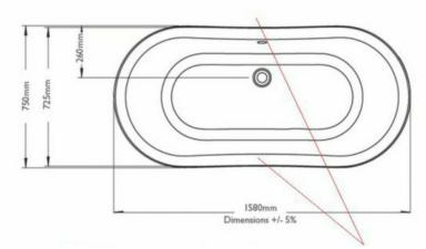
NB: the rim on the long sides bend inwards by approximately 20mm in the middle, so there will be a gap between the centre of the bath and the wall
