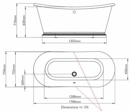
NB: the rim on the long sides bend inwards by approximately 20mm in the middle, so there will be a gap between the centre of the bath and the wall
