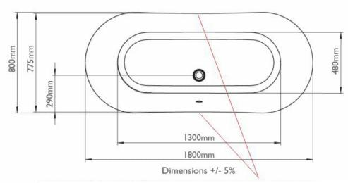
NB: the rim on the long sides bend inwards by approximately 20mm in the middle, so there will be a gap between the centre of the bath and the wall
